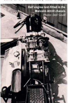
housing and other redundant protruding casting infringements were cut away in order to facilitate the installation in the chassis.
