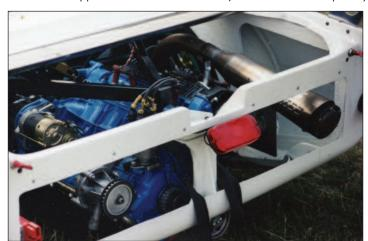
The car was fitted out with a lot of single-seater technology using centre lock wheels, multiple wishbones, exotic steering, damper and spring systems, etc and ran with a variety Jack Knight transaxles bolted to 1,200 cc Imp race engines.
