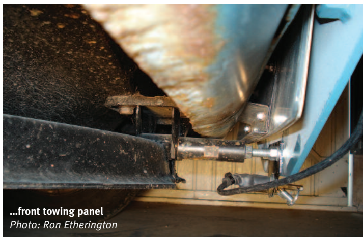
Modified front wishbone mounting ready to accept... Photo: Ron Etherington
