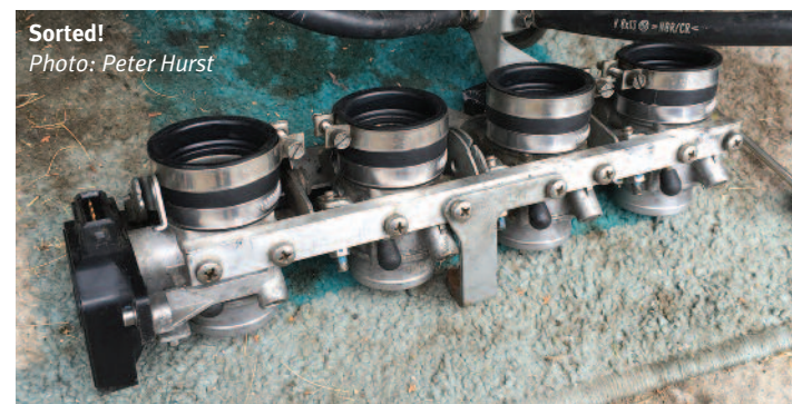
Perished throttle body rubber seals cause of rough running. Cheap and easy to replace Photo: Peter Hurst
