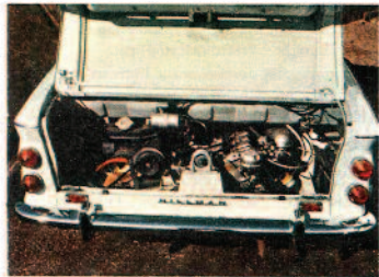
Scotland's Hillman has its engine at the back, neatly angled for ease of access. With Britain out of the Common Market, selling the Imp abroad will be an even tougher business
