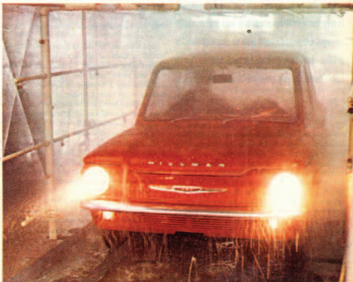
From all angles, including the underside, each Imp is spray-tested for body leaks by powerful waterjets as it comes off the assembly line
